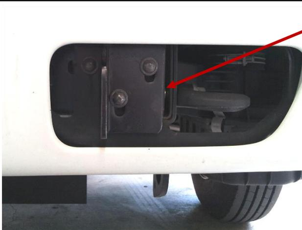
FIT MOUNT BRACKETS TO VEHICLE USING ORIGINAL BOLTS
