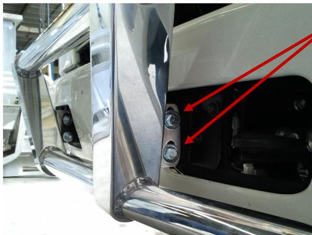
FIT NUDGE BAR TO OUTSIDE OF MOUNTS AND SECURE USING 1 1/4" x 3/8" BOLTS, FLAT WASHERS, SPRING WASHERS AND NUTS
