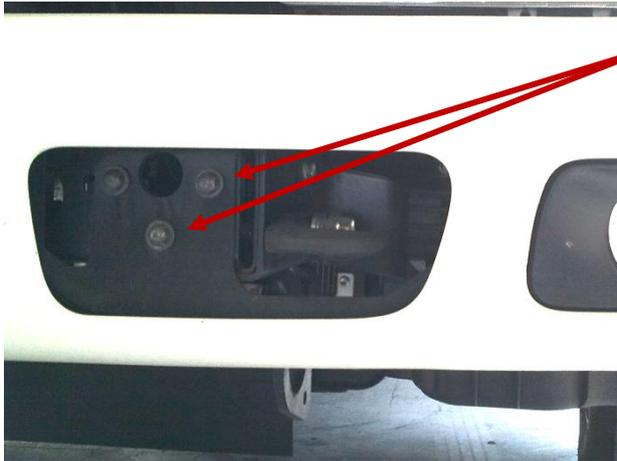
REMOVE TWO (2) OUTER BUMPER RETAINING BOLTS FROM FRONT OF BUMPER ON BOTH DRIVER AND PASSENGER SIDE
