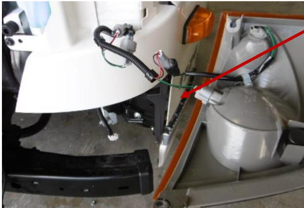
OPEN BONNET AND REMOVE INDICATOR FASTENERS
