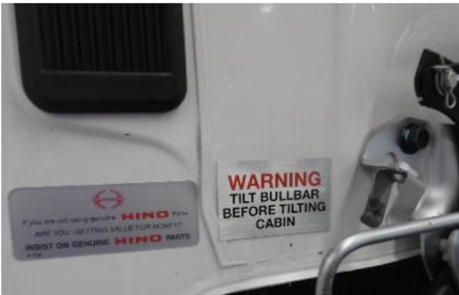
FIT TILT BULLBAR WARNING STICKER TO PASSENGER SIDE REAR OF CABIN NEAR TILT LEVER
