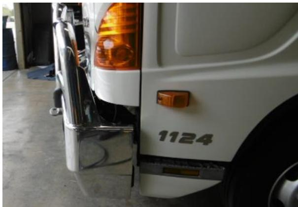
ALIGN THE BULLBAR WITH THE VEHICLE AND TIGHTEN ALL CHASSIS MOUNT FASTENERS FULLY
