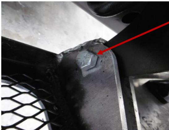
LIFT BULLBAR INTO POSITION, ALIGN EYEBOLTS AND LIGHTLY FASTEN
