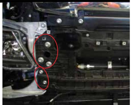
17mm and 12mm bolts shown with headlight corner plastics removed for photo
