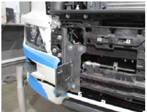
Fitted photo taken after trimming grille backing in next step.
