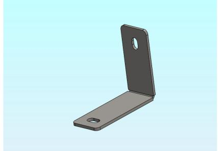
Figure 4 - Underbelly splash guard brackets
