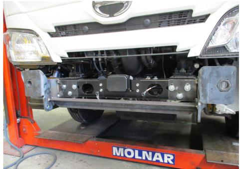
NOTE: Rear hole has captive nut on passenger side.
