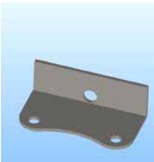
Figure 6 - Fog light mounting brackets
